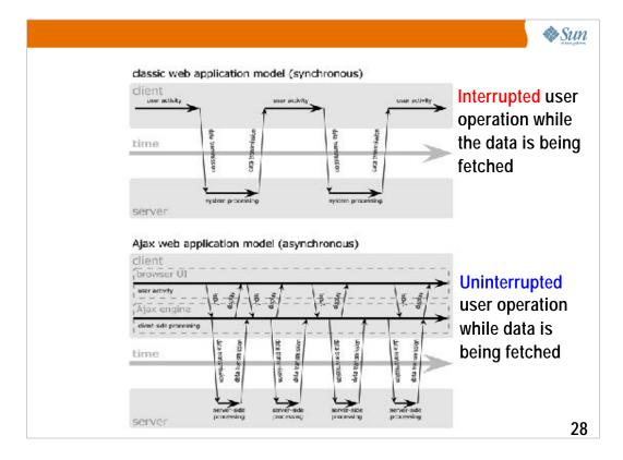
I assume some of you have seen this picture before. This picture compares the user interaction models of conventional web application in the top half of the slide against AJAX-fied web application in the bottom part of the slide.
